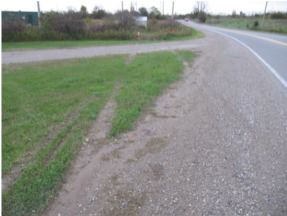
Figure 7: Tire marks in the grass of the east roadside show how the southbound vehicle progressed to line of bushes and wire fence in the background.
