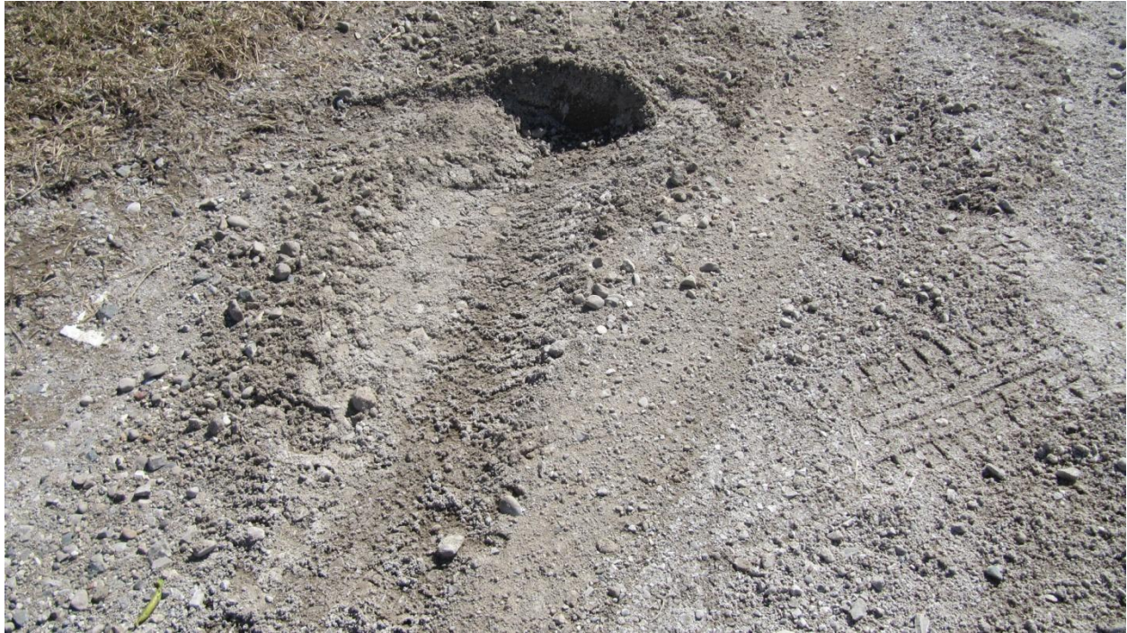
Figure 36: A close up view of one of the ends of the tire marks shows how the sliding tire comes a halt a the mound of earth and then there is a tire print progressing to the left where the rolling tire begins to move after coming to a halt as the driver moves the vehicle to exit the site.
