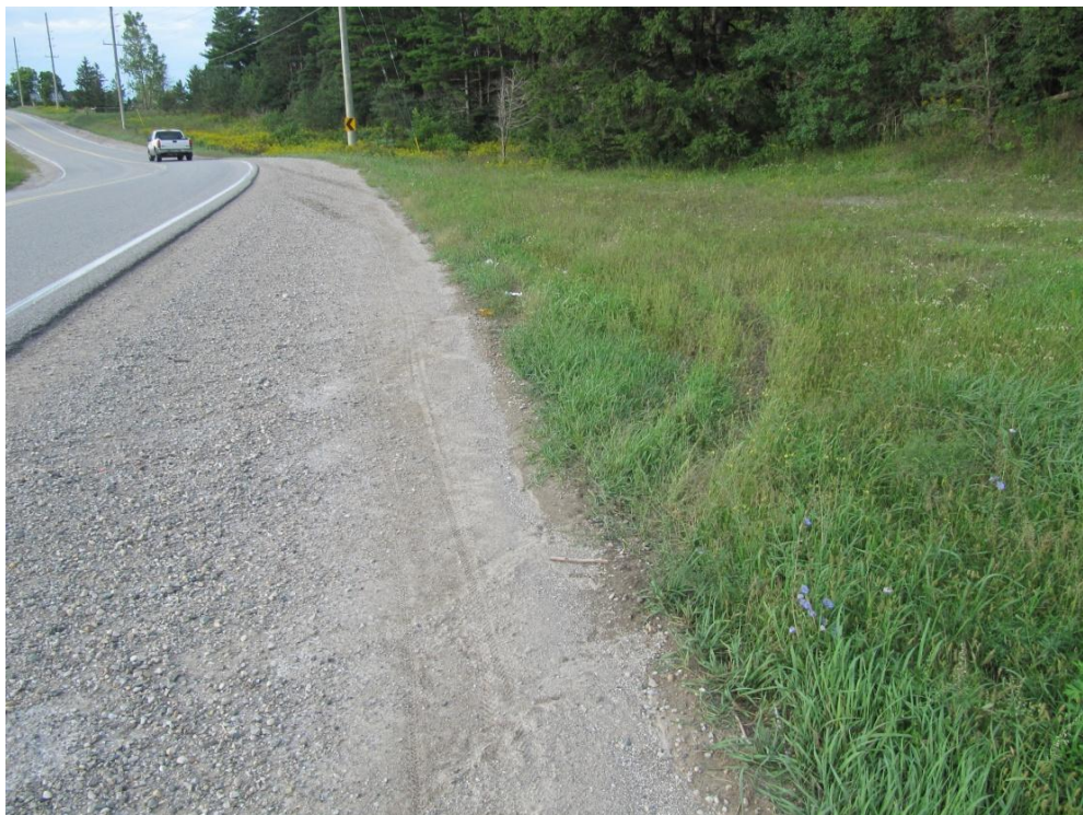
Figure 32: View, looking north, at the tire marks as the rotating vehicle passes through the gravel shoulder in the foreground on its return back onto the road surface.
