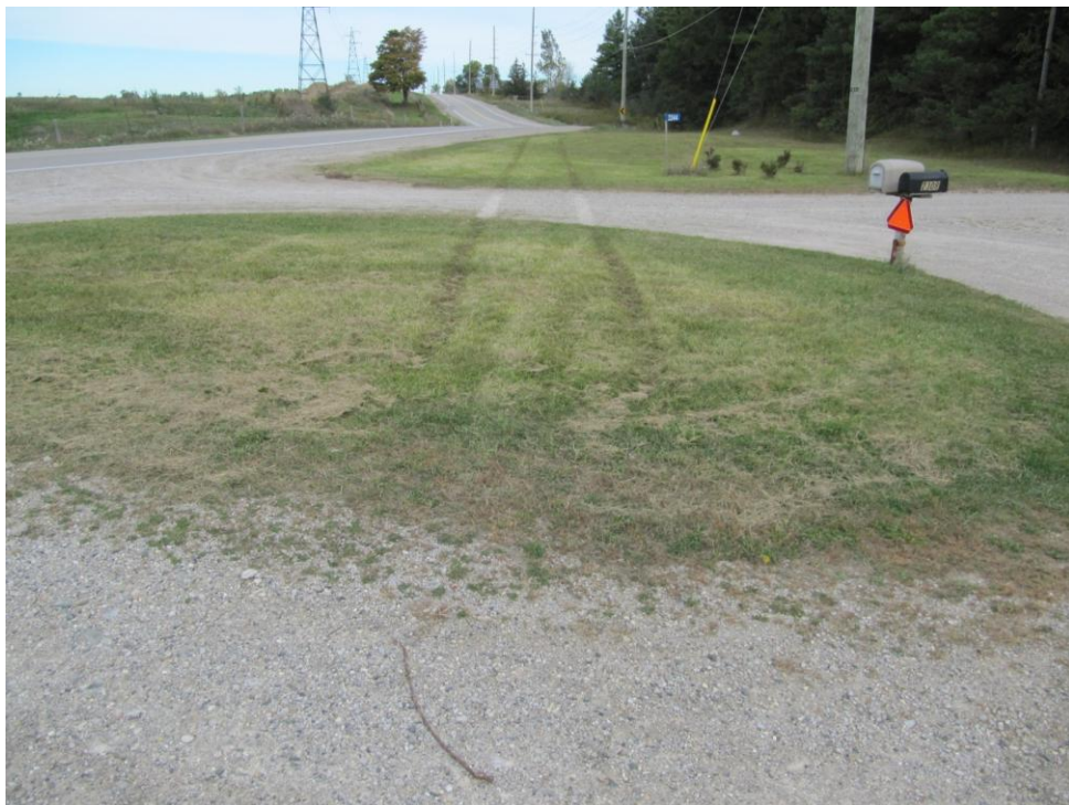
Figure 29: View, looking north, showing that the tire marks terminate in the grass in the foreground and no additional marks are visible in the gravel in the foreground.
