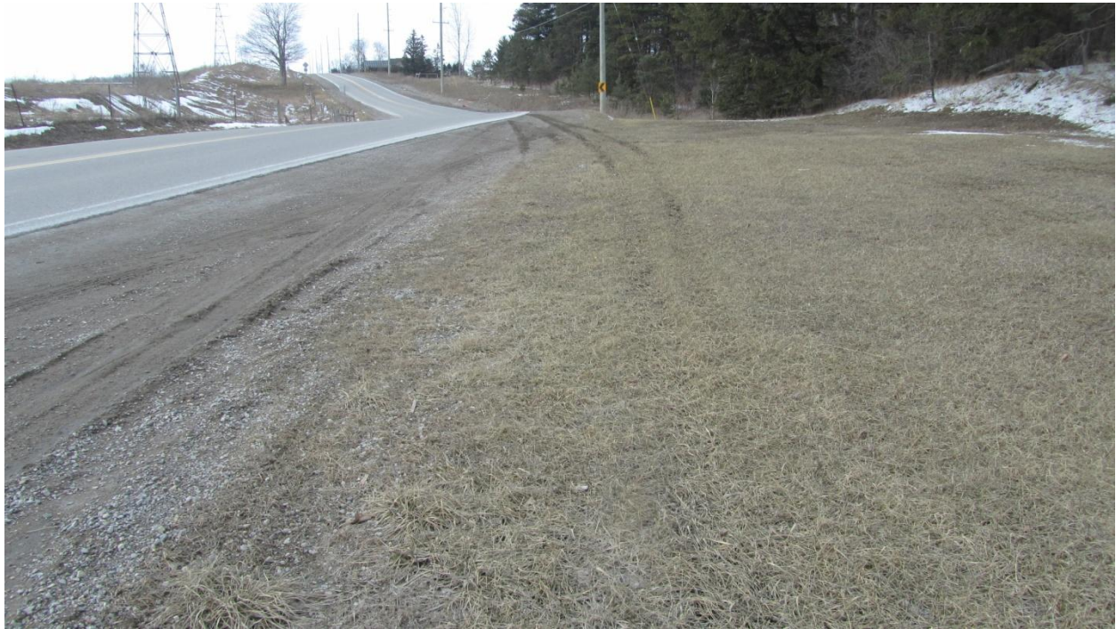
Figure 46: View, looking north, at the tire marks of the southbound vehicle approaching the camera.
