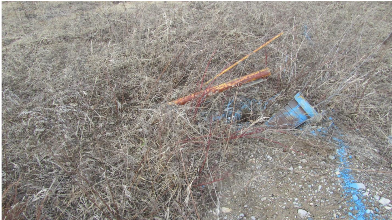
Figure 56: A side-view of the stuck pipe. The southbound vehicle was travelling from the left to the right and pushed the pipe and yellow pole to a horizontal position.
