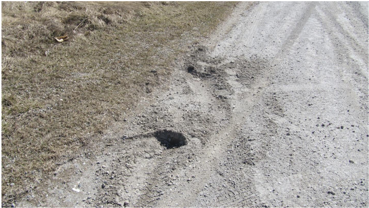
Figure 35: View showing the tire marks where the vehicle's tires gouge into the gravel as the tires slide sideways and then two mounds of gravel/earth are created at the precise location where the wheels came to stop.
