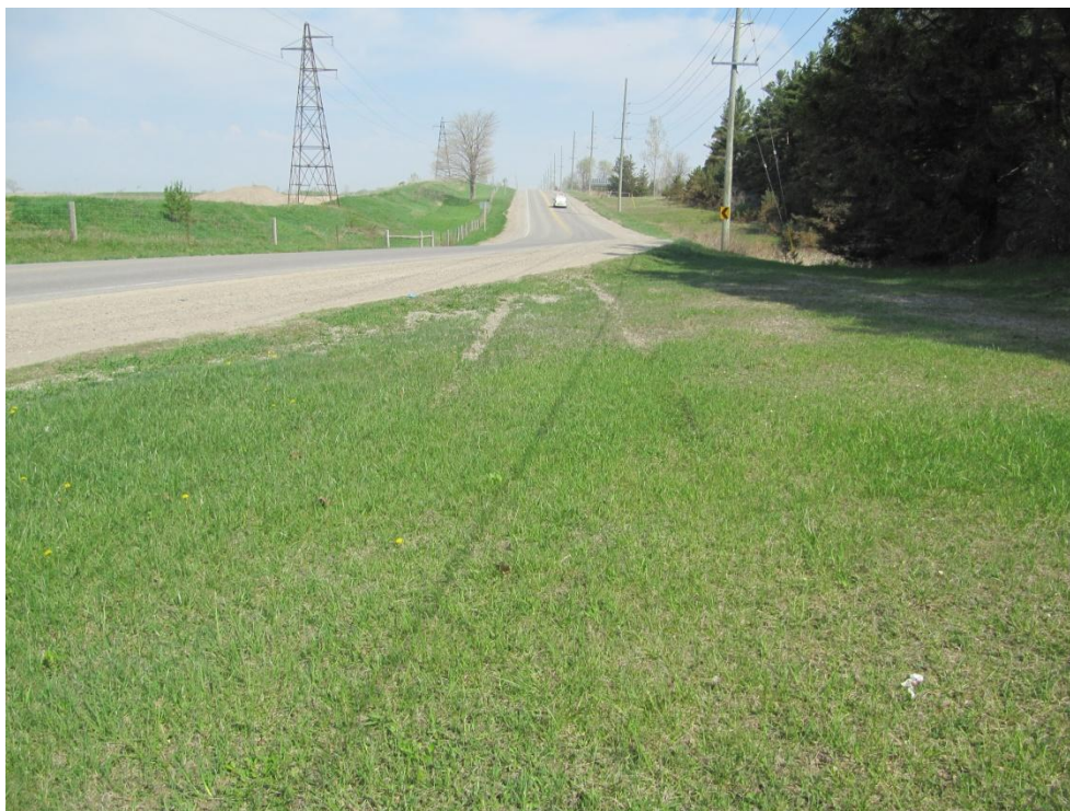
Figure 20: View, looking north, at the tire marks exiting onto the grass. The marks are no longer visible in the foreground indicating the deterioration of the evidence but also suggesting that the vehicle mass might have been partially lifted due to its speed.
