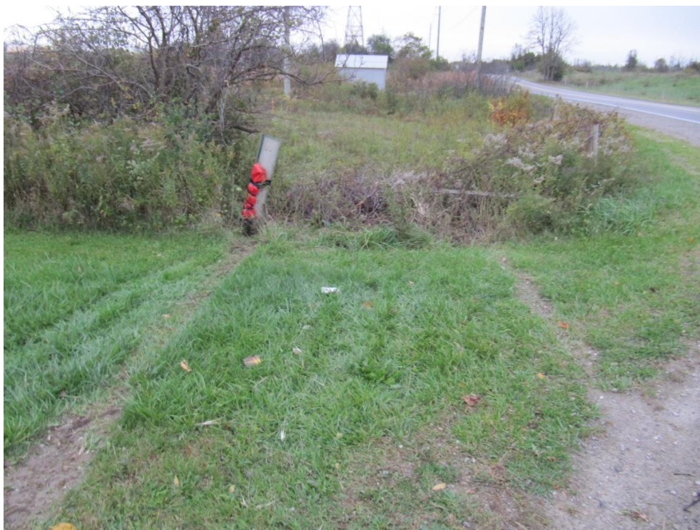
Figure 8: Tire marks show how the southbound vehicle drove into the bushes and fence and passed through these obstacles.
