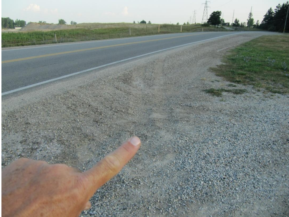
Figure 16: View, looking northward, showing the tire marks in the gravel as we look back to where the vehicle first exited the road surface.
