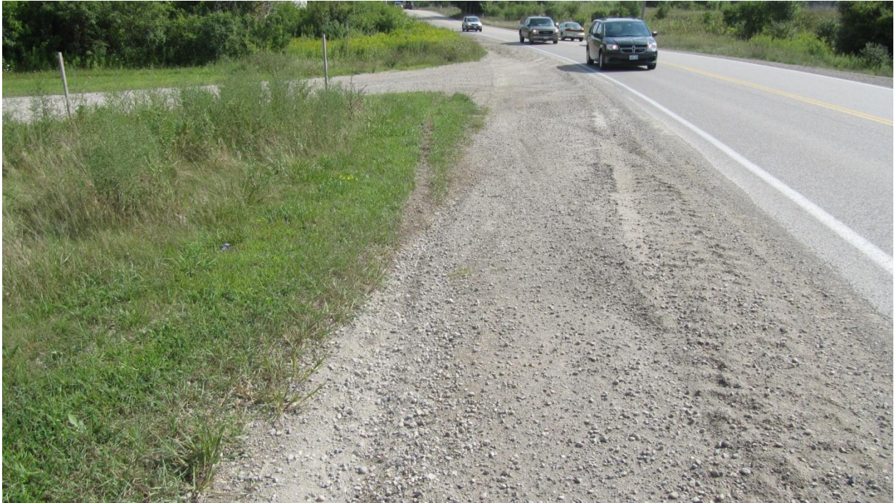
Figure 40: View, looking south, at the yaw marks created on the east shoulder and roadside.
