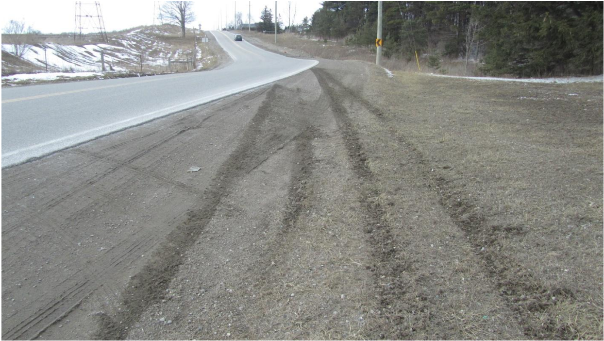
Figure 43: View, looking north, at the tire marks of the southbound vehicle as it enters the east shoulder.
