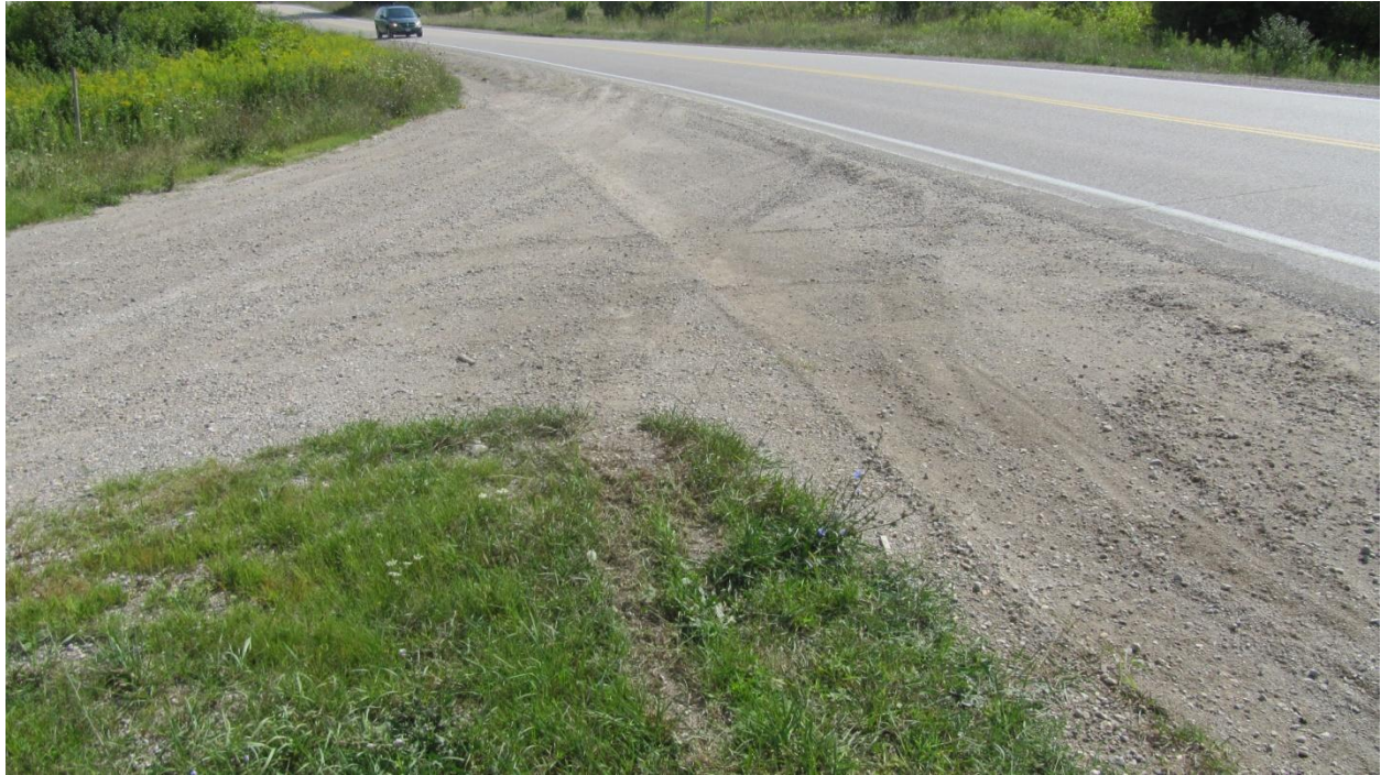
Figure 42: The physical evidence of the curved tire marks suggests that the driver may have regained control of the vehicle without stopping and then continued to re-enter the road to proceed southbound again.
