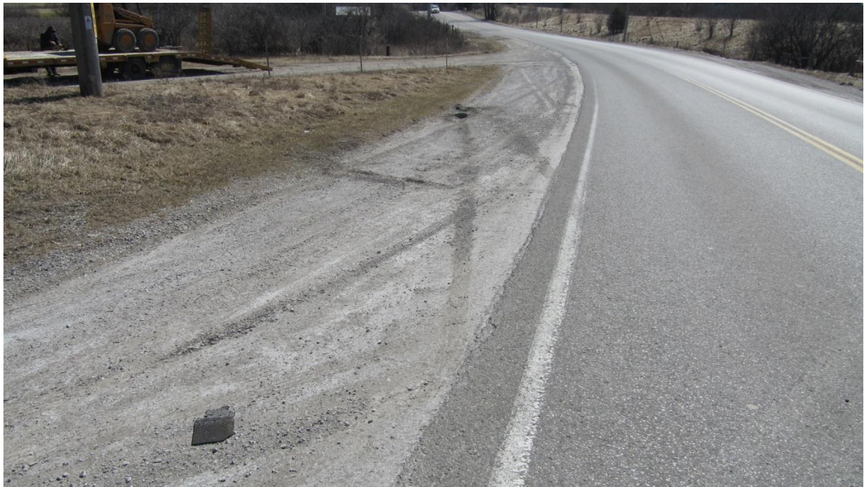
Figure 34: View, looking south, at the yaw marks on the east shoulder indicating that the vehicle is rotating counter-clockwise. Additional tire marks exist because, after the vehicle came to a halt it then accelerated away and left the site.
