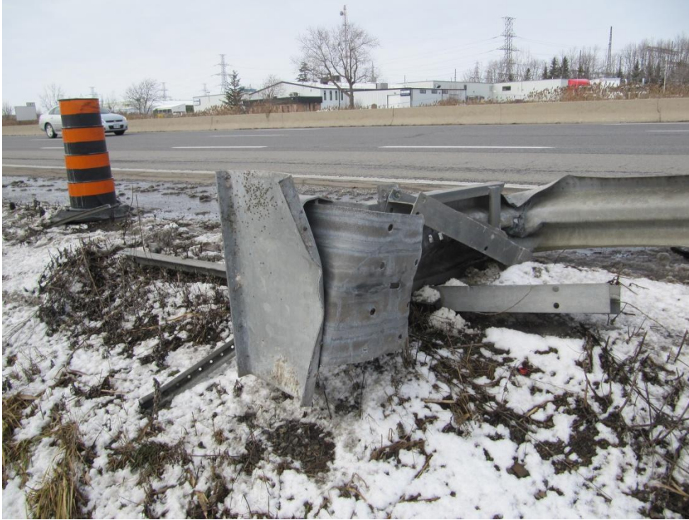
Figure 4: View of the deformed end plate of the ET-Plus terminal and the short length of the rail that has passed through the throat of the ET-Plus terminal.
