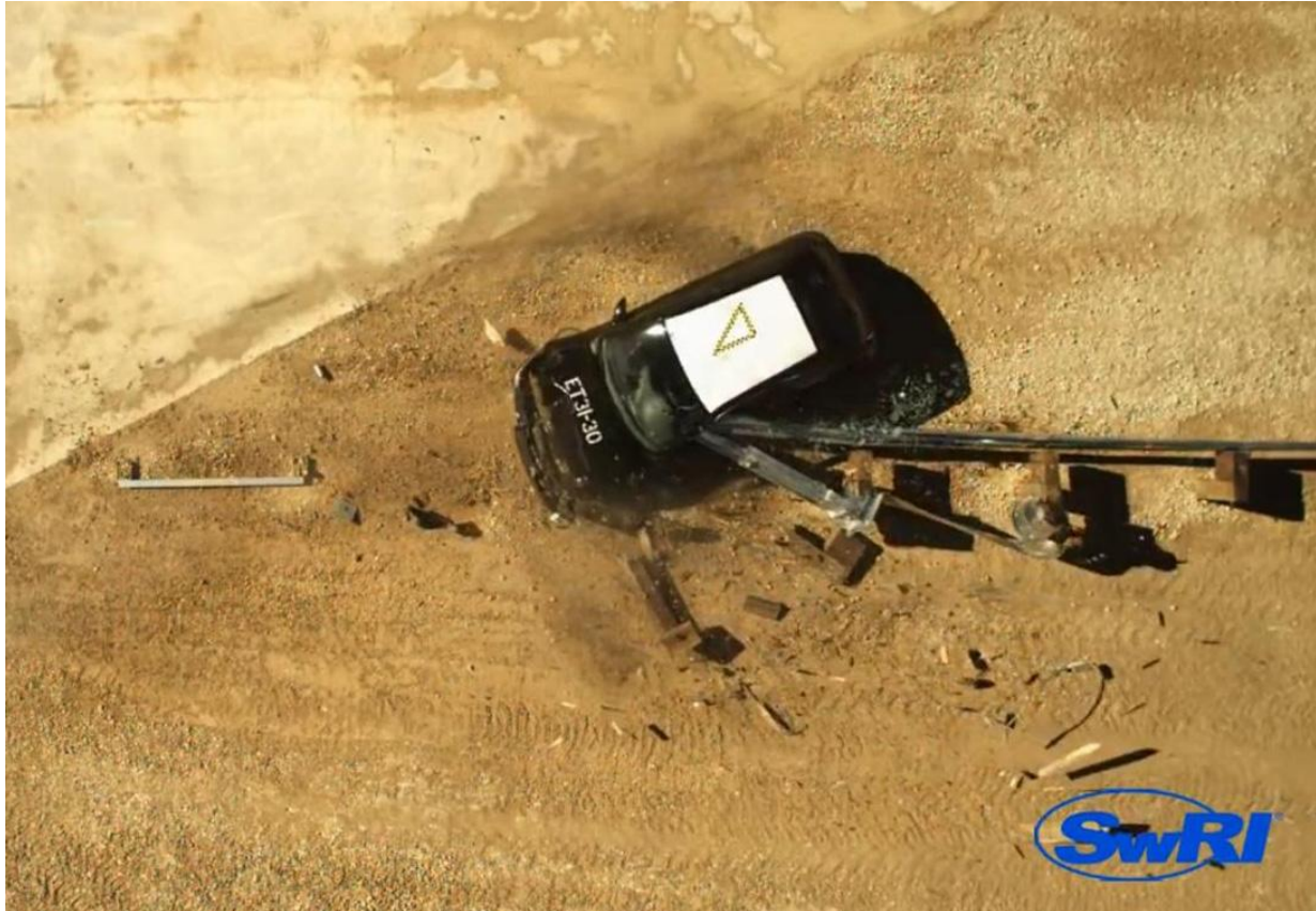
Figure 34: As the Metro continues to rotate the rail forms a spear that penetrates the driver's interior.
