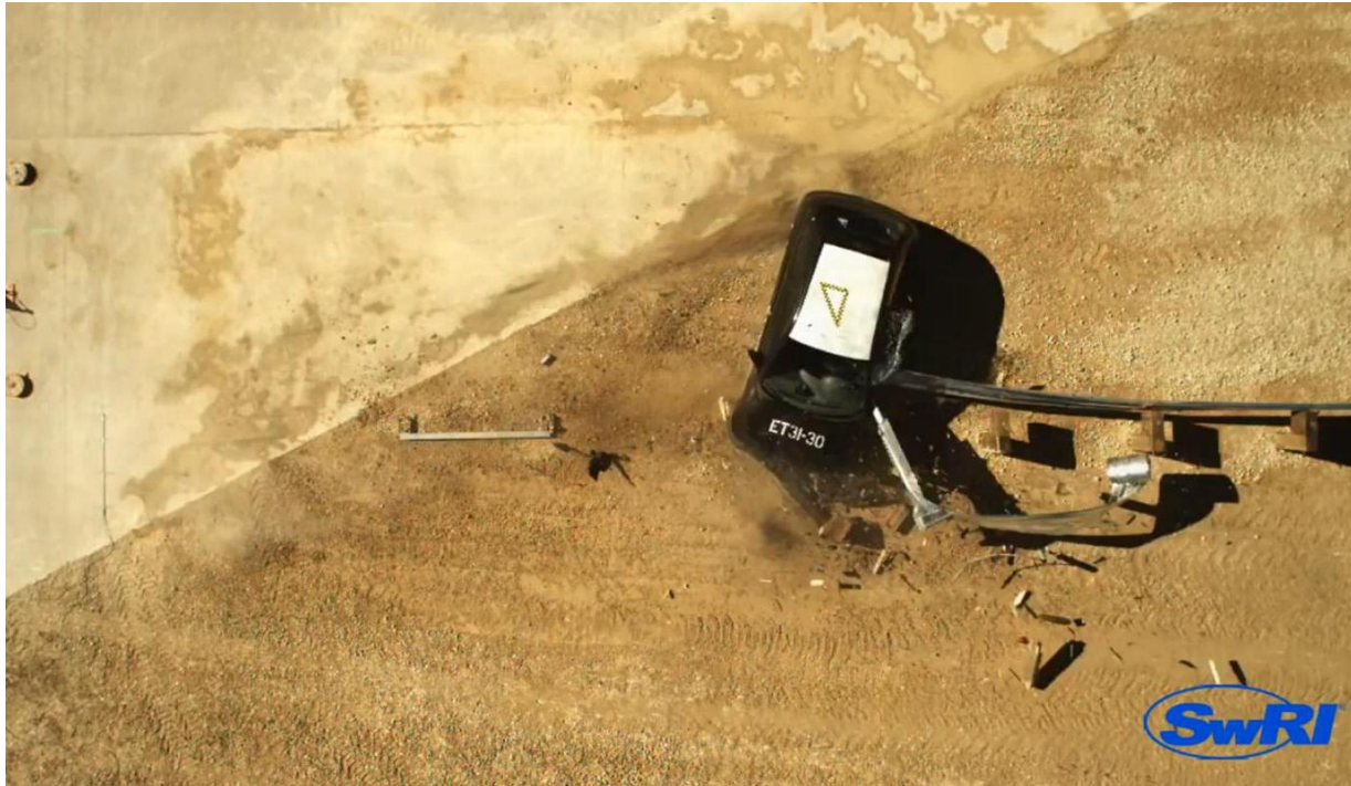
Figure 33: The rail doubles over just behind the terminal forming a spear that penetrates into the driver's door.
