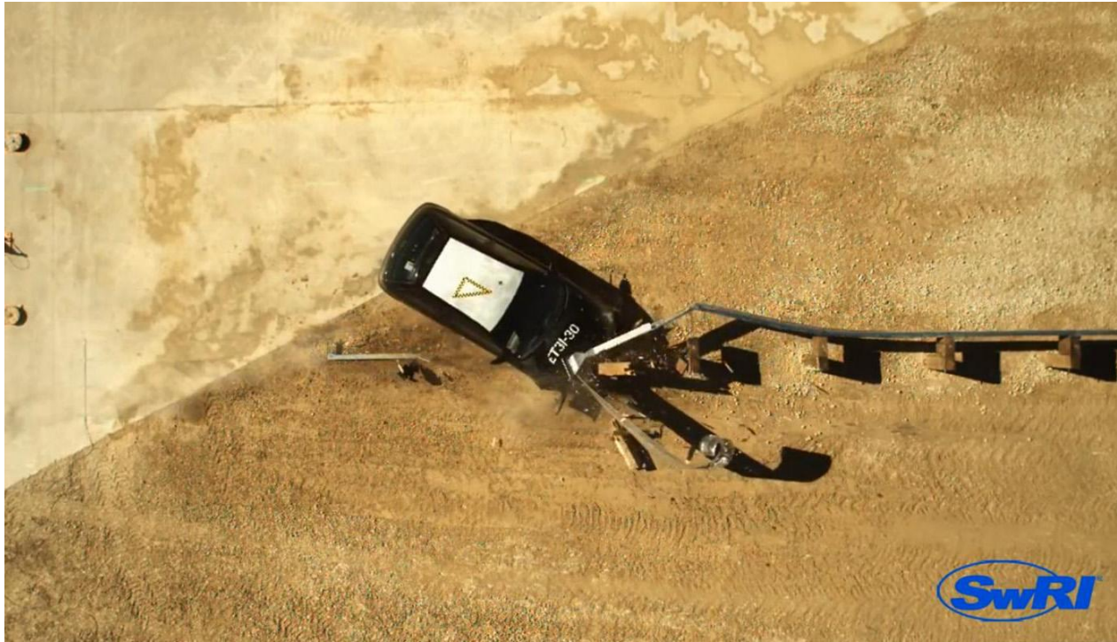
Figure 31: The rail begins to buckle the Metro rotates.
