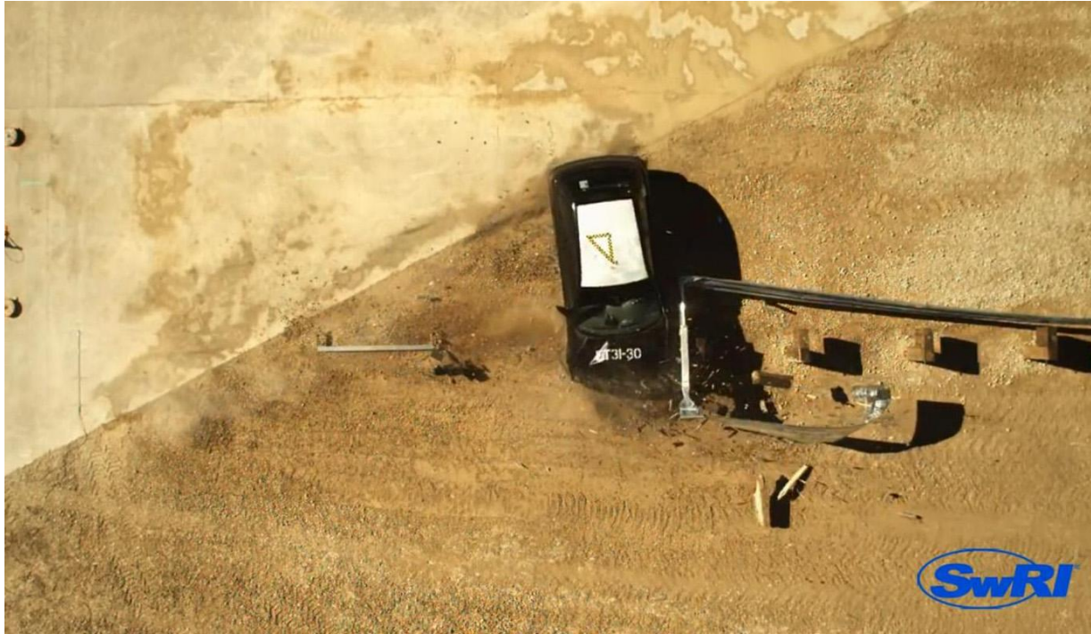
Figure 32: The rail continues to buckle as the Metro continues to rotate.
