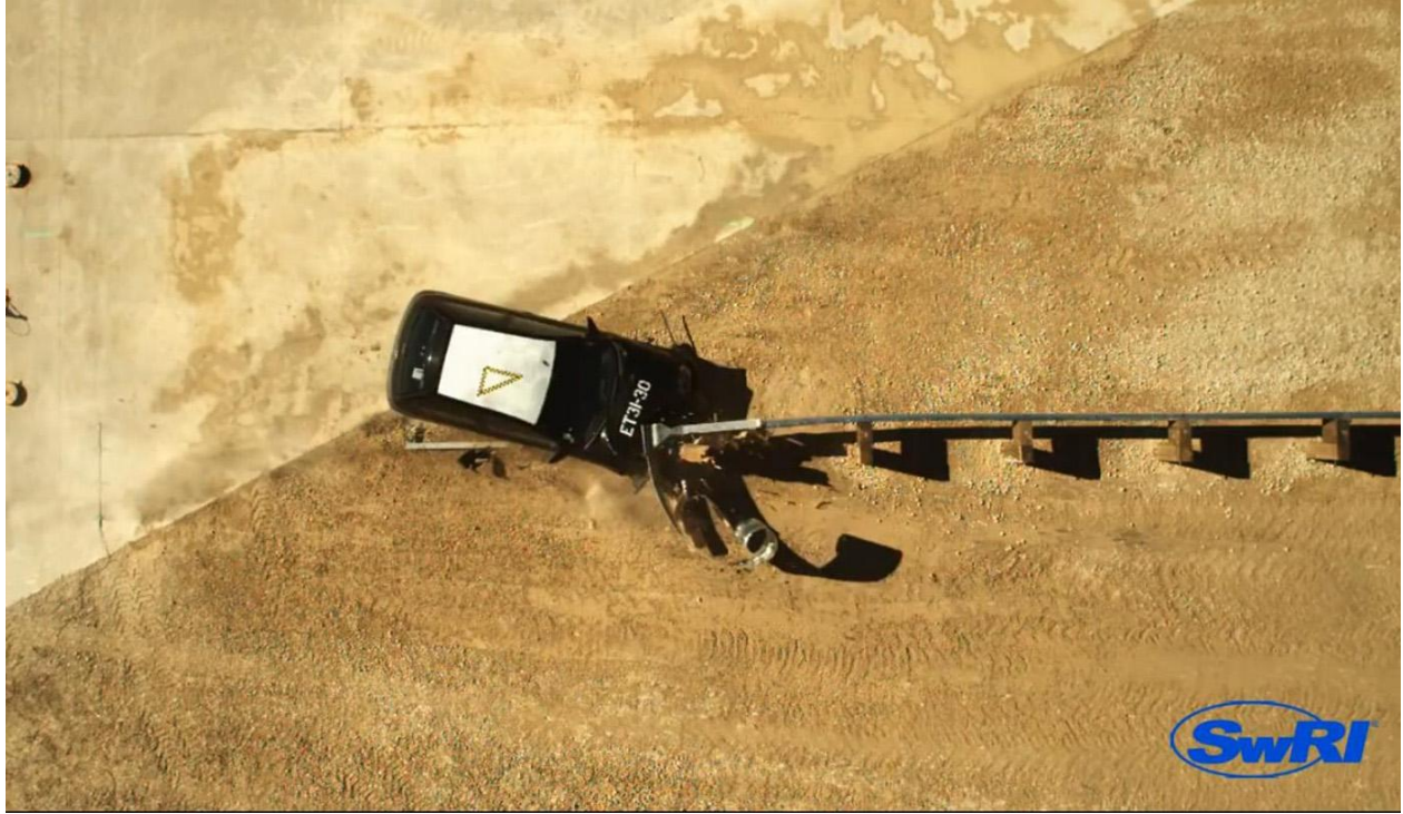
Figure 30: View of the Metro after it has travelled a considerable distance and has caused a considerable amount of rail to be extruded through the terminal head.
