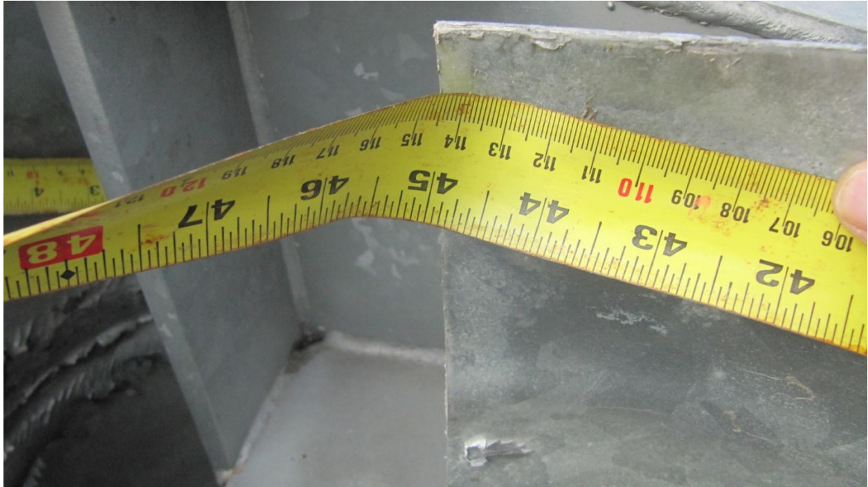
Figure 17: View of the end result of the measurement method shown in Figures 15 and 16, indicating that 114 centimetres of the rail had been squeezed through the throat of the terminal.
