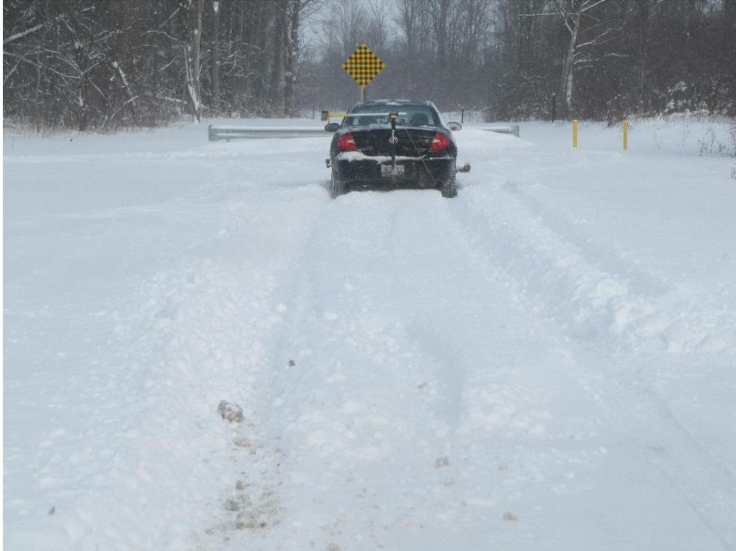
Figure 2: Resultant snow disbursement following braking Test #8 in deep snow.
