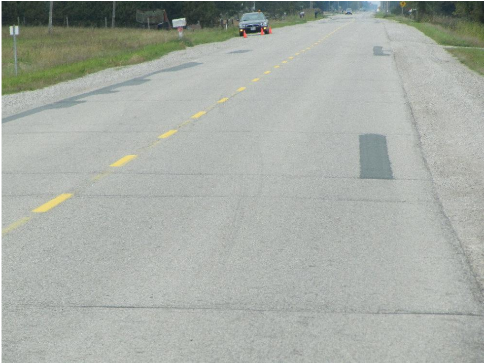
Figure 16: Westward view showing how a longer focal length (zooming in) causes the compression of the dark transfers from the tire marks and therefore makes them more visible.
