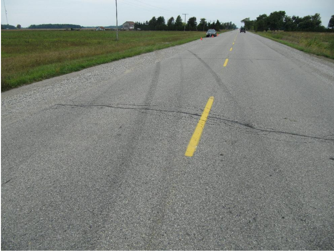
Figure 11: View, looking west, at the yaw marks travelling from the westbound lane, across the eastbound lane and into the south ditch.
