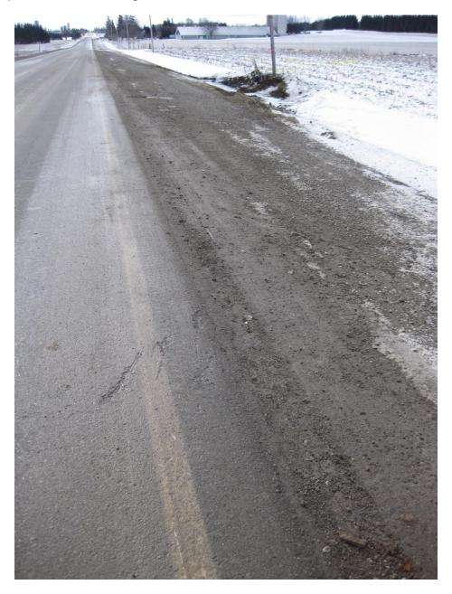
The character of these gouges is typical of what you might see at an area of impact. It clearly shows that, after impact, the very large mass of the Tanker truck continued to move southward, off the road surface, and into the west ditch where it struck the utility pole.
