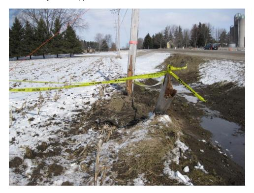
The photo below shows that slope and you can see the tire marks that indicate how the tanker truck moved off the road and toward the impact with the pole. You can also see my vehicle and cones in the background to orientate where this evidence is located.
