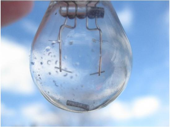
Let us recall that when a light is "on" the tungsten becomes soft and when an impact force occurs "near" its location it will stretch. When a light is "off" the tungsten is brittle and if an impact force occurs "near" its location it may fracture. Just to give you more information, below is another view of the bulb. Look closely at the sides of the glass. Enough said.
