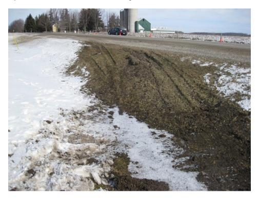
This evidence should clearly indicate to you that the truck was moving southward as it left the road, not northward, as reported by the news media. For comparison, we can look at the area of the road just south of the pole impact as shown in the photo below.
