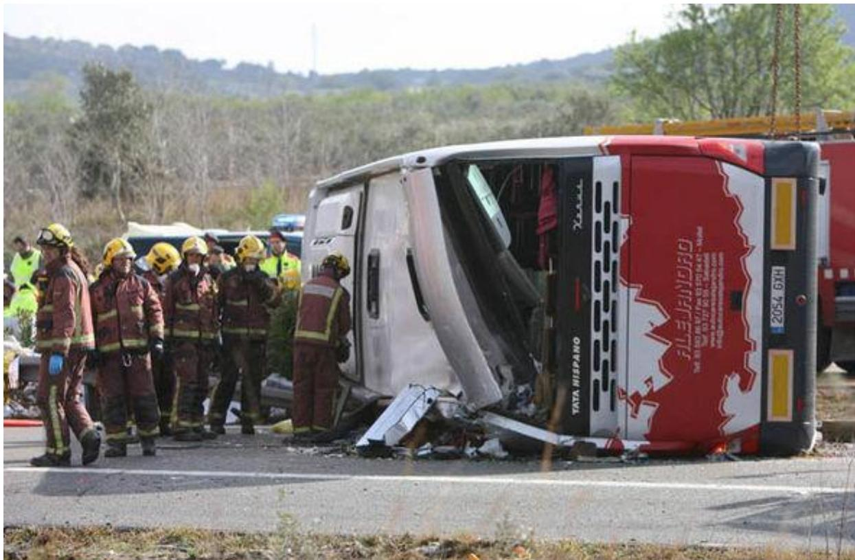
Figure 3: View of the crush exhibited to the rear corner of the roof of the bus.
