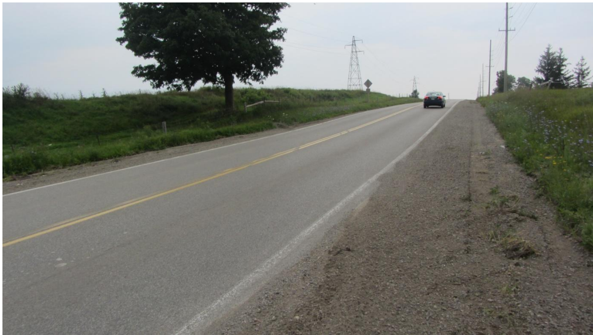
Figure 40: View looking north from the north end of the yaw marks in the foreground as the rotating, northbound vehicle returns to the road surface. At the centre-line, in the centre of the view, are some black transfers of rubber with striations within them indicating that these are from the continued yaw mark produced by the northbound vehicle. The vehicle eventually comes to rest on the west shoulder adjacent to the tree in the background.
