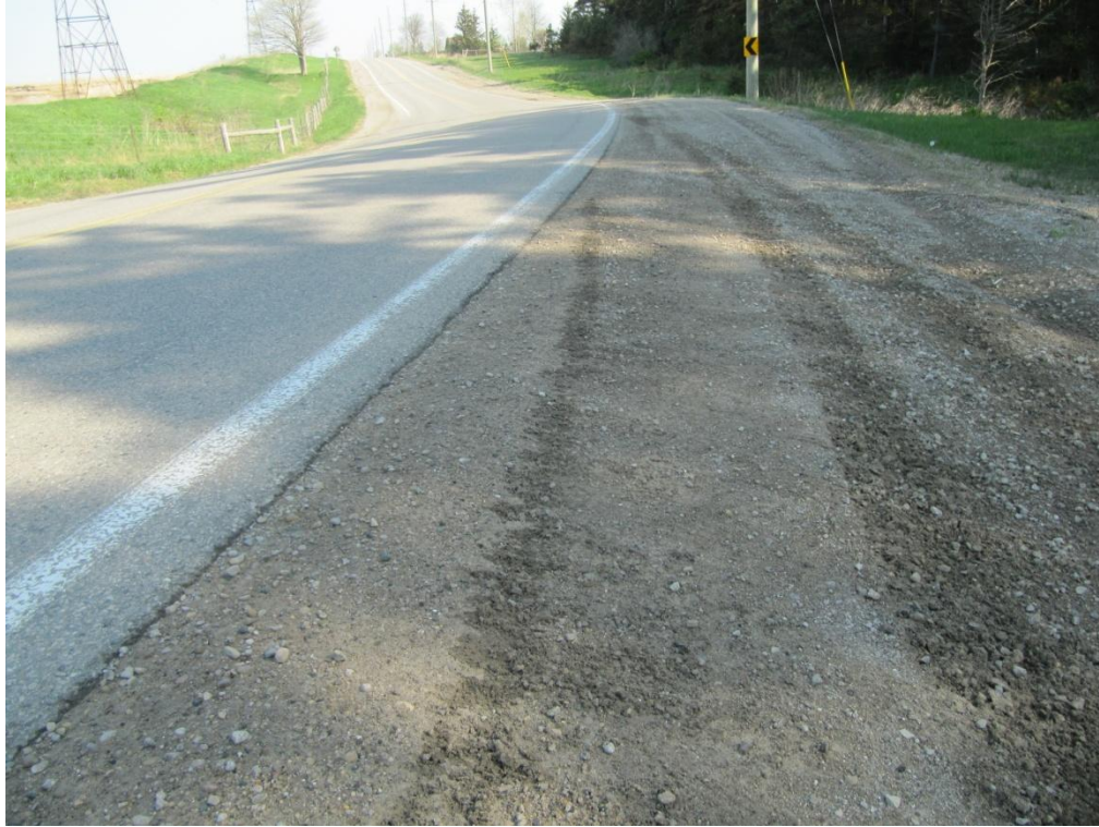
Figure 35: View looking north along the east shoulder showing the yaw marks as a southbound vehicle travelled toward the camera while rotating clockwise.
