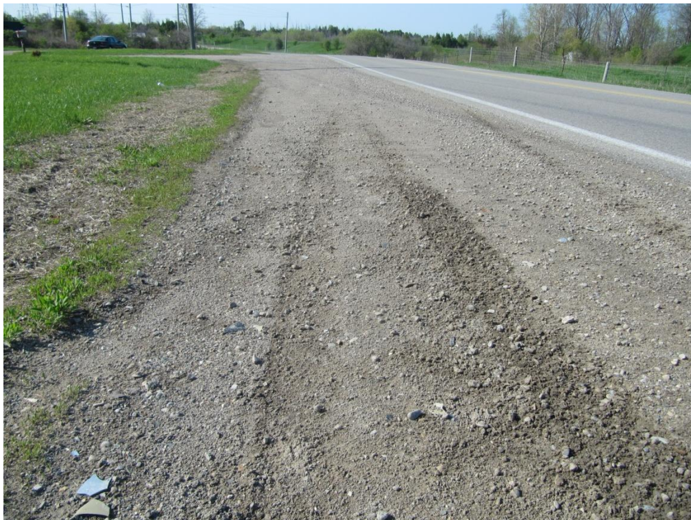
Figure 36: View looking south along the east shoulder showing how the yaw marks fade out as the driver regains control of the vehicle and continues southbound back onto the road.
