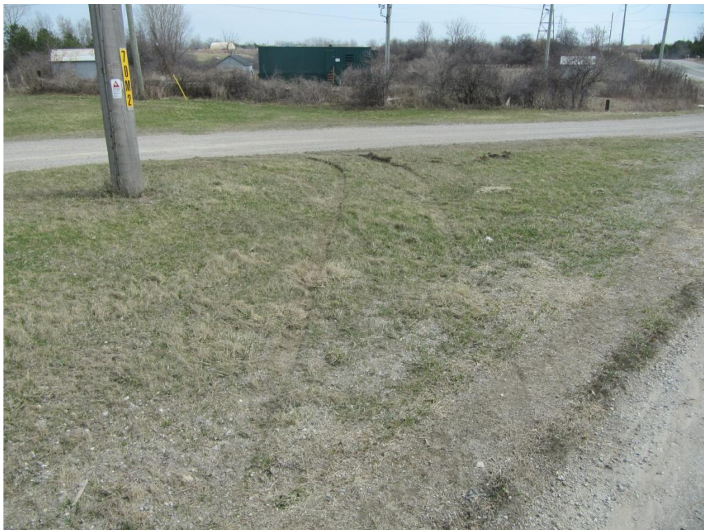
Figure 33: View of tire marks on the east roadside showing an exit from the road by a southbound vehicle which is then steering hard to the left under high acceleration in the background.
