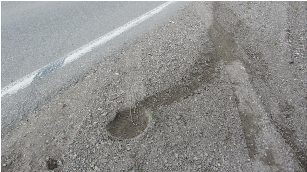
Figure 44: Close-up view of the tire marks at the final rest position of the northbound vehicle. The tire marks show how the vehicle slid to rest and then tread marks shows how the vehicle then exited and drove away.
