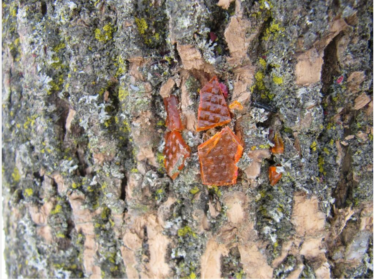
View of Orange Lens Material Clinging to the Bark of the Struck Tree.
