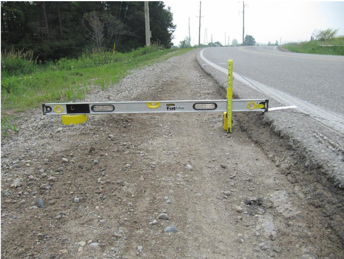
View of procedure used to measure edge drop off on Clarke Road north of Fanshawe Park Road (Circa Aug 2011).
